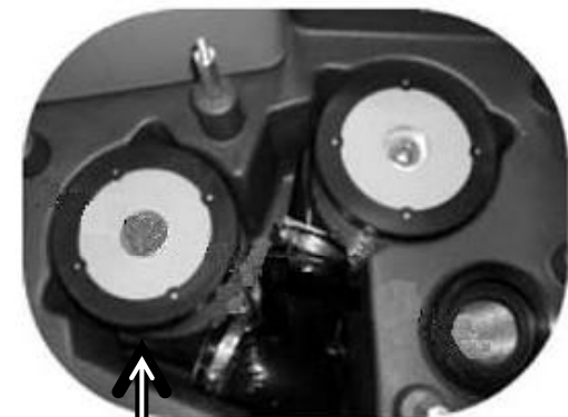
↑ ↑ Float/Screen ↑ ↑ Vacuum Motors
