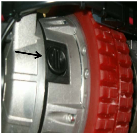
Chassis Drive Motor Carbon Brush Locations (under caps) Carbon Brushes Part # 241400-2
